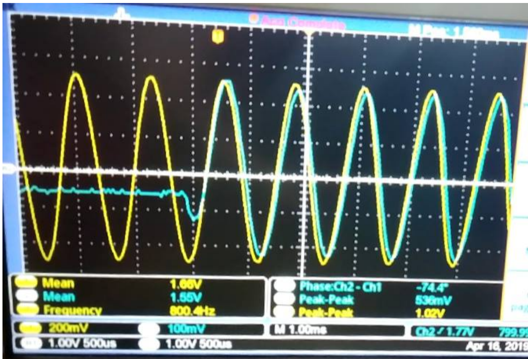
Figure 8: Current and Forcing Function, with Current set as zero initially
